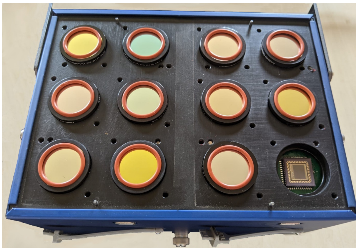
Figure 4: Opened Tetracam micro-MCA. From left to right and top to bottom, spectral sensors of the wavelengths 550 \pm 10 nm, 670 \pm 10 nm, 840 \pm 10 nm, 900 \pm 20 nm, 570 \pm 10 nm, 700 \pm 10 nm, 860 \pm 10 nm, 950 \pm 40 nm, 780 \pm 10 nm, 450 \pm 40 nm, 720 \pm 10 nm, and incident light sensor (bottom right corner).
